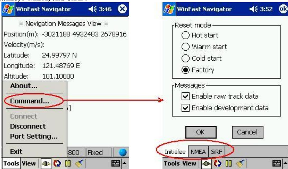
The **Initialize**, **NMEA**, and **SiRF** configuration screens under **Command** are as shown in the figures below:
